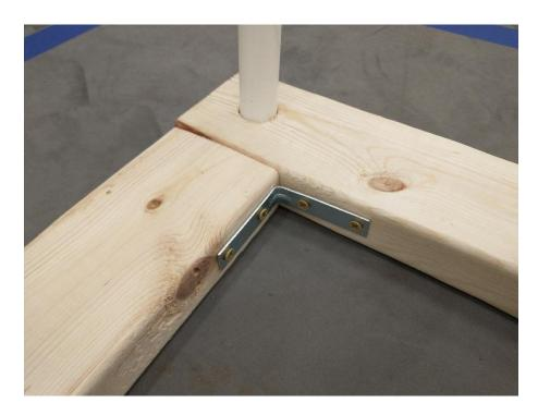
The holes for the scoring poles are drilled with a 1" diameter spade bit, and are placed at the intersection of the centerline of each side piece.
