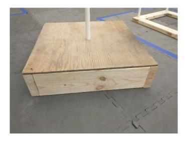
The hole for the scoring pole is drilled in the center of the top cover. A support strut is placed along the bottom of the base frame, with a hole to help keep the scoring pole aligned.
