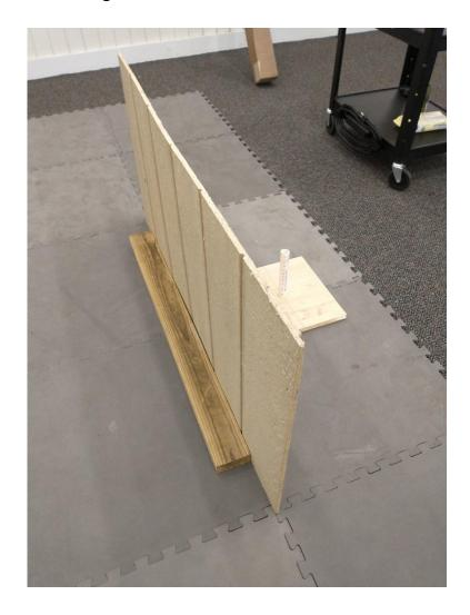
The screen is made from a 24" by 48" piece of  $\frac{1}{2}$  plywood. A standard 2X4 is attached with screws to the bottom of the screen front for stability. A 12" by 18" piece of  $\frac{1}{2}$  plywood is attached with screws to the bottom of the screen back to act as a support for the 6" scoring pole and for stability.
