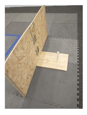
The hole for the scoring pole is drilled 12" from the screen and centered on the width of the base support plywood.
