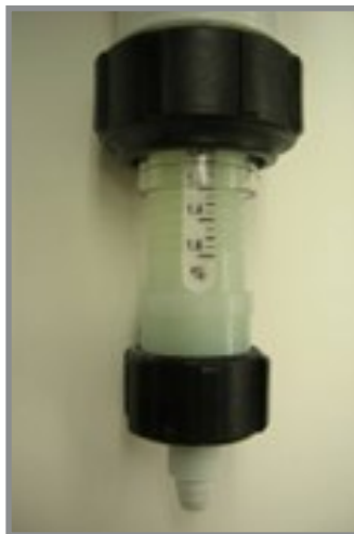
Figure 4. The injector proportioner allows you to adjust your injection rate by either % or by ratio.
