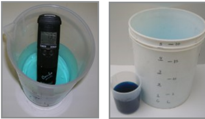
Figure 6. (Left) Calibration by electrical conductivity (EC) requires an EC meter. Each fertilizer type has a specific electrical conductivity based on the desired concentration. (Right) The dilution ratio calibration is the most simple method. It requires only a measuring container and a receiving bucket, each with measured graduations.
