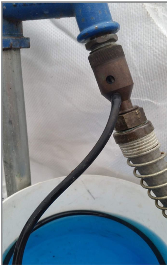
Figure 1. The most simple venturi injector. A Hozon® venturi injector delivers a soluble concentrate at 1:16 dilution ratio at a minimum of 35 psi.
